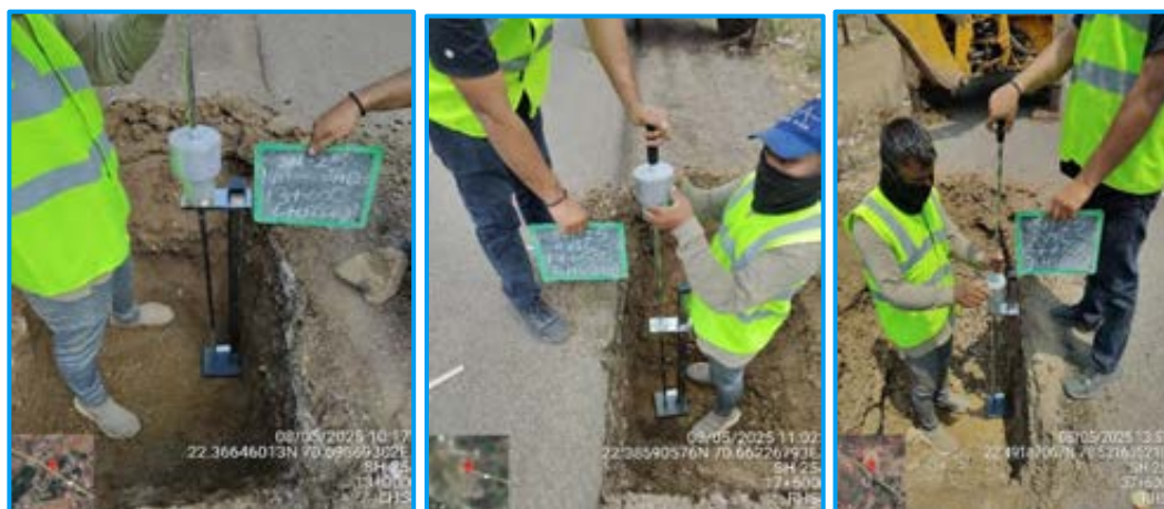
Figure 8-1: Field Investigations photographs of DCP-CBR
