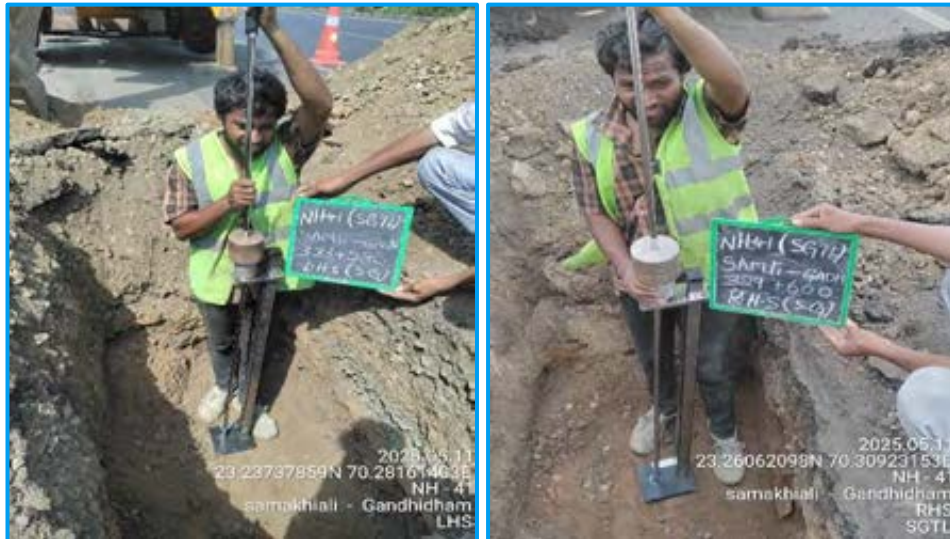
Figure 8-1: Field Investigations photographs of DCP-CBR
