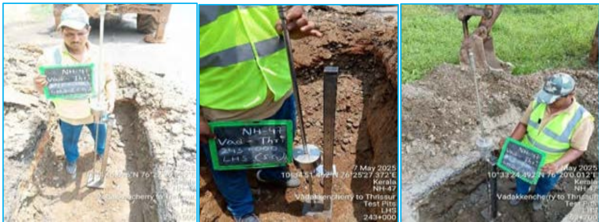
Figure 8-1: Field Investigations photographs of DCP-CBR
